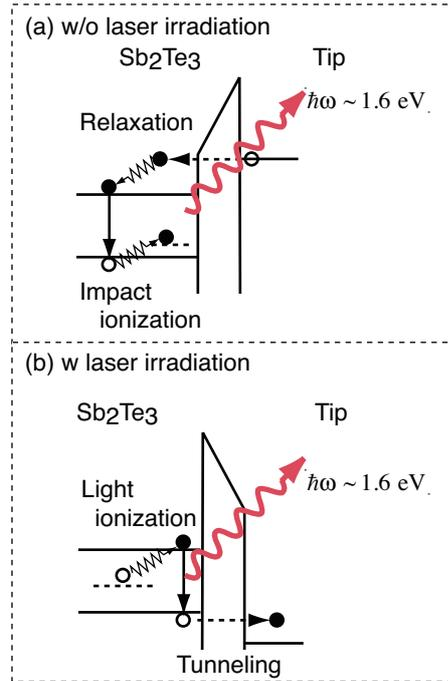
Fig. 3 STM light emission mechanisms operated when the laser irradiation is (a) off and (b) on.
