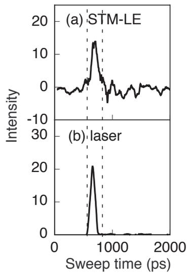
Fig. 4 Temporal behaviors of (a) STM light emission from the W tip-Au sample gap irradiated with the picosecond laser pulses and (b) the picosecond laser pulses themselves. These spectra were measured with a streak camera operated in a mode whose temporal resolution is 100 picoseconds.
