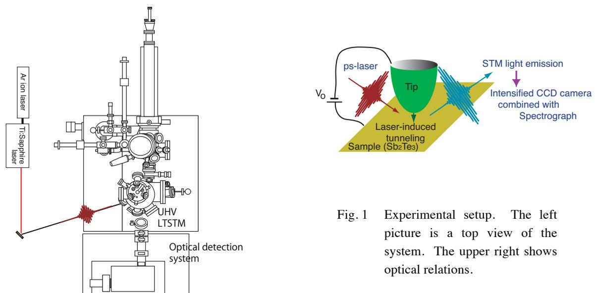
Fig. 1 Experimental setup. The left picture is a top view of the system. The upper right shows optical relations.
