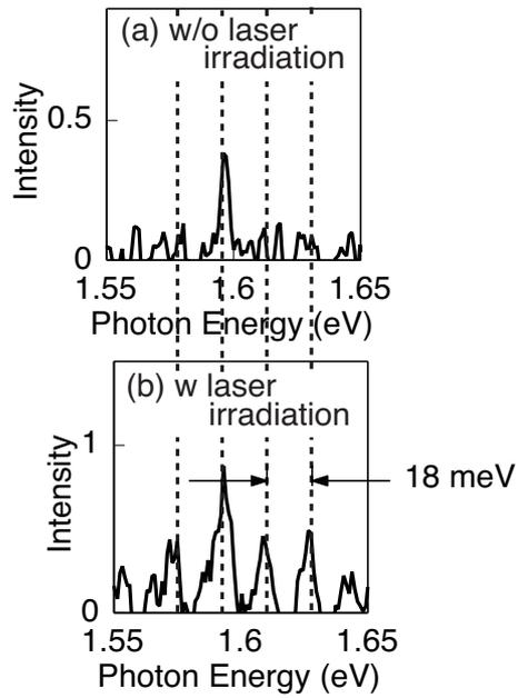
Fig. 2 STM light emission spectra observed when the laser irradiation is (a) off and (b) on. multiple peaks are seen only in (b).
